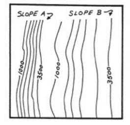
The distance between contours indicates the steepness of a slope; close spacing denotes steep slopes; wide spacing denotes gentle slope.
