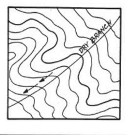
Contours tend to parallel streams and have an M-shape just above stream junctions.
