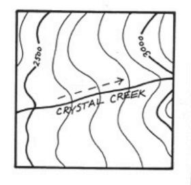
The U's made by contours crossing ridge lines point down the stream.
