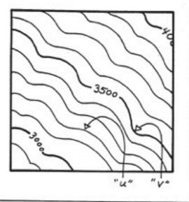
The V's formed by contours crossing a stream point upstream.
